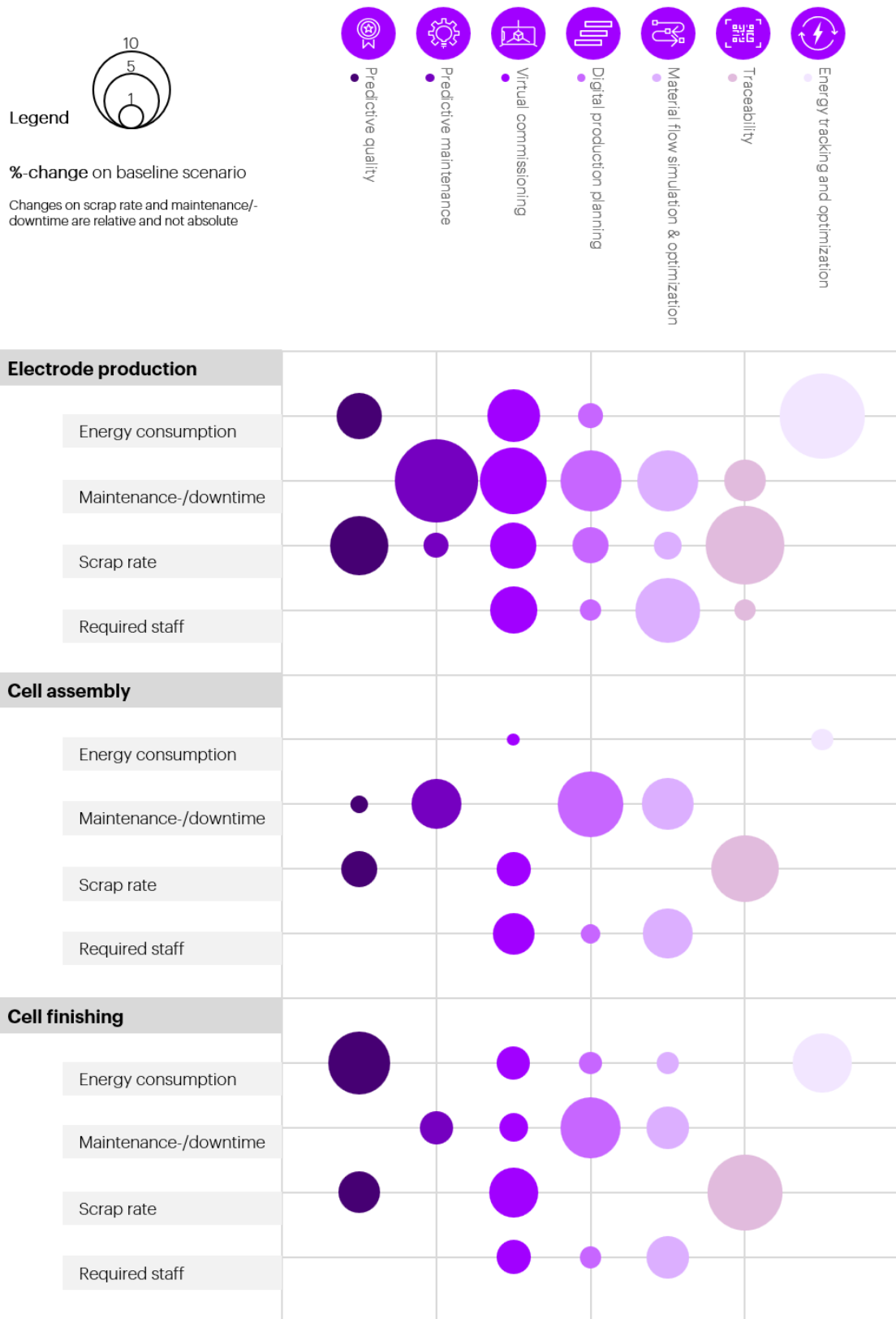
Figure 5: In an online survey, 63 participants were tasked with evaluating the impact of seven selected use cases on key performance indicators (KPIs) related to cost drivers. Participants expressed their input as a relative improvement compared to a baseline scenario for all cell manufacturing steps, spanning from mixing to end-of-life (EOL) cell testing. The mean results based on process step input are presented aggregated into the three main segments of cell production: electrode production, cell assembly, and cell finishing.
